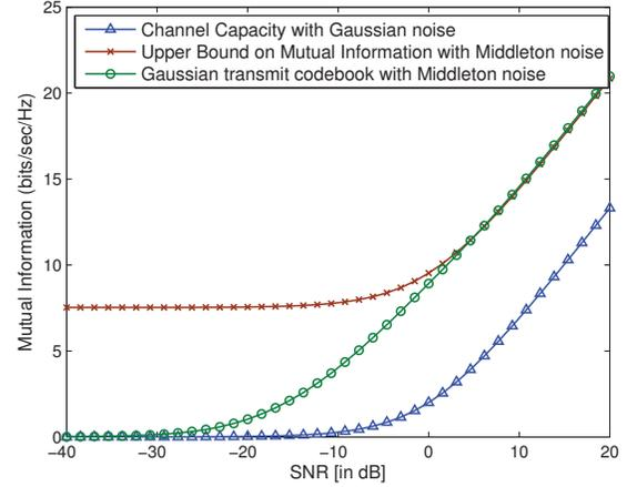
Fig. 1. Mutual information in the presence of Gaussian and bivariate Middleton Class A noise with parameters  $A = 0.1$ ,  $\Gamma_1 = 0.01$ ,  $\Gamma_2 = 0.1$  and  $\kappa = 0.4$  for a  $2 \times 2$  MIMO system.
