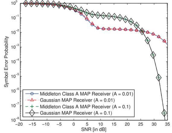
Fig. 2. Symbol error probability with MAP decoding rule for Gaussian and Middleton Class A noise under additive bivariate Middleton Class A noise with parameters  $\Gamma_1 = 0.01$ ,  $\Gamma_2 = 0.1$  and  $\kappa = 0.4$ . The error probability curves for Gaussian and Middleton Class A noise MAP receivers are indistinguishably close in this figure.
