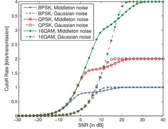
Fig. 4. Cutoff Rate with MAP decoding MIMO receiver in presence of Gaussian and bivariate Middleton Class A noise with parameters  $A = 0.1$ ,  $\Gamma_1 = 0.01$ ,  $\Gamma_2 = 0.1$  and  $\kappa = 0.4$ .
