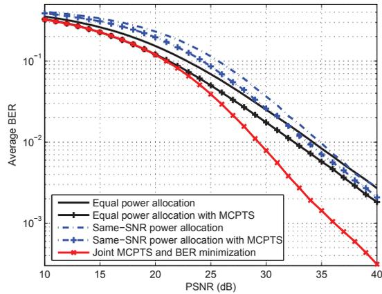
**Fig. 3.** Average BER versus PSNR curves for  $M = 8$  multi-channel OFDM systems.
