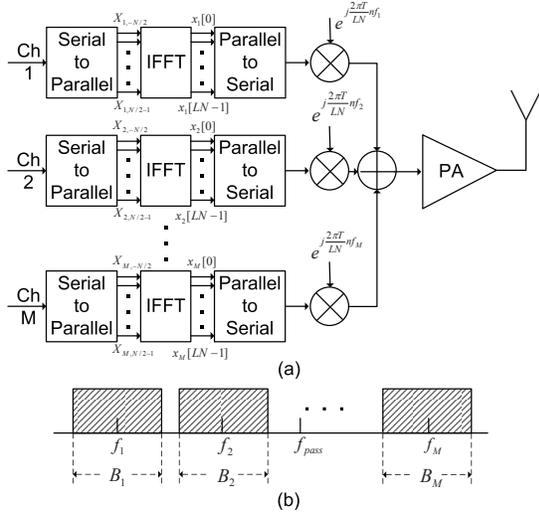
**Fig. 1.** The (a) structure and (b) frequency spectrum diagram of the multi-channel OFDM base station.
