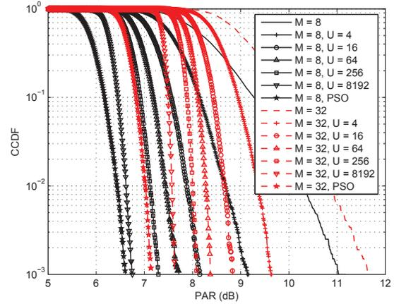
**Fig. 2.** CCDF curves of the PAR of the original and MCPTS multi-channel OFDM signals for different numbers of channels ( $M = 8, 32$ ) and numbers of phase sequences ( $U = 4, 16, 64, 256, 8192$ ) as well as the PSO method.
