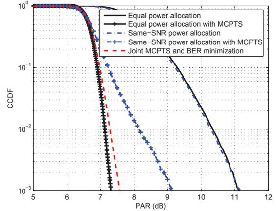
**Fig. 4.** CCDF curves of the PAR for  $M = 8$  multi-channel OFDM systems.
