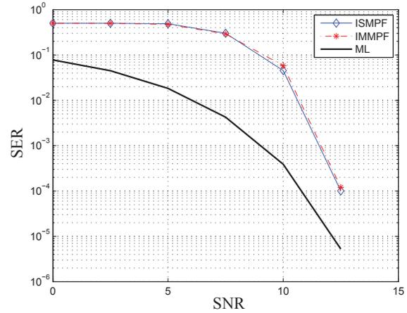
Fig. 2. The SER vs. SNR for unknown  $\alpha$  at  $F_d T_s = 0.005$  and  $N = M = T = 2$ .
