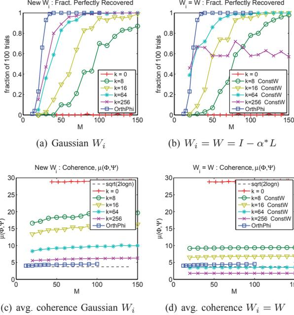
Fig. 2. Impact of weights strategies, random weights (left) vs. constant optimal consensus weights (right), at various mixing levels,  $k$ . The corresponding coherences of sensing and propagation matrices are shown below.
