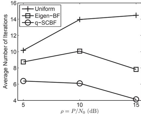
**Fig. 1.** Convergence speed of optimum multiuser beamforming solution with different initial beamformers
