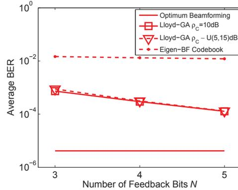
**Fig. 3.** Average BER over MIMO channels with limited feedback at  $\rho = 10$ dB
