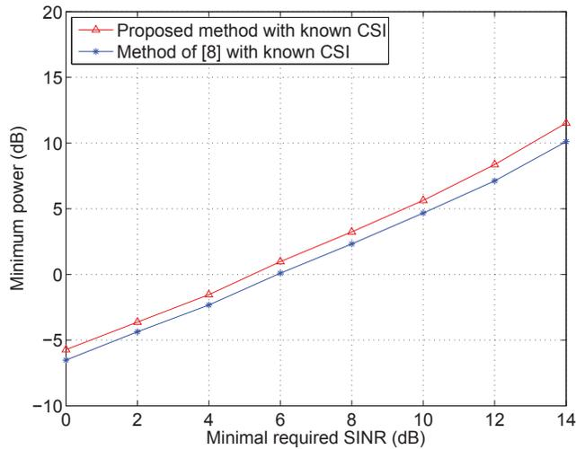
**Fig. 2.** Total relay transmitted power versus minimal required SINR.  $K = 2$ .
