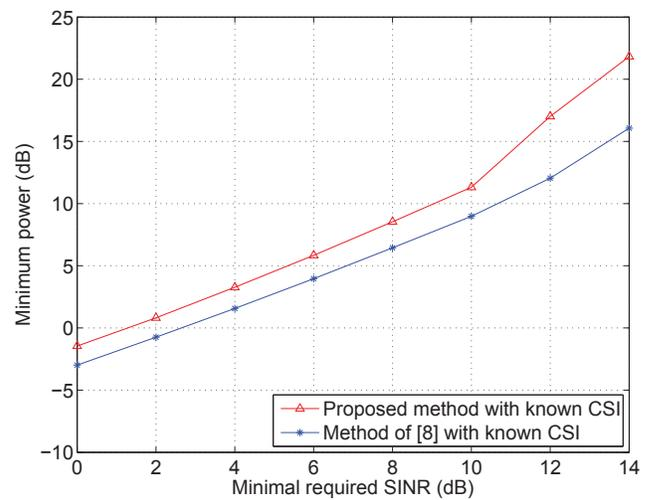
**Fig. 3.** Total relay transmitted power versus minimal required SINR.  $K = 3$ .
