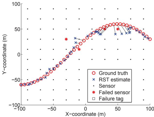
**Fig. 2.** Undetected sensor failures that cause erroneous tracking results
