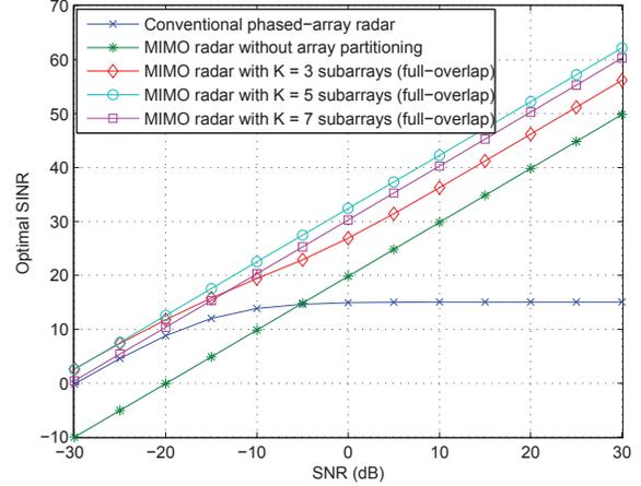
Fig. 1. Optimal output SINR versus SNR; first example.
