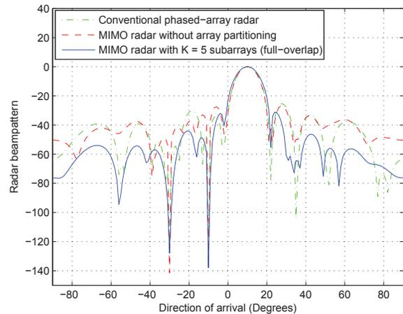
**Fig. 3.** MIMO radar beampattern.
