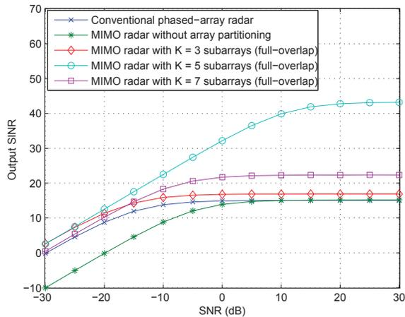
**Fig. 2.** Output SINR versus SNR, second example
