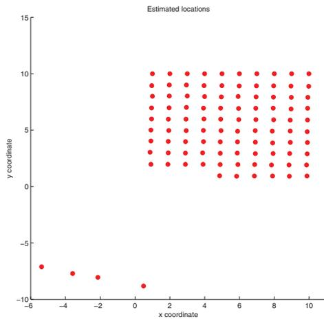
**Fig. 2.** Position estimation using the proposed algorithm. There are 4 outlier nodes and 10 reference nodes (top row). The outliers do not influence the location estimates of the other nodes.
