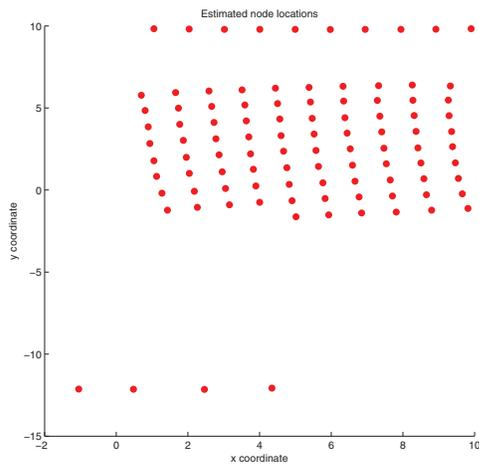
**Fig. 3.** Position estimation using least squares localization. There are 4 outlier nodes and 10 reference nodes (top row). The outliers greatly influence the location estimates.
