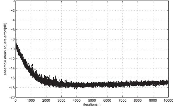
Figure 4: Learning curve of the proposed method using the algorithm in (17).
