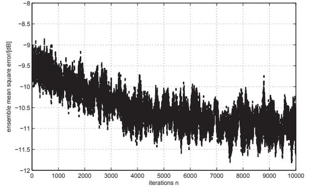
Figure 5: Learning curve of the generalised sidelobe canceller based on the same uniform linear array.
