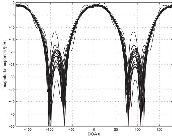
Figure 6: The resultant beam pattern of the proposed method for the frequency range  $\Omega \in [0.5\pi; \pi]$ .
