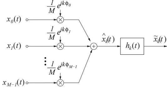
Figure 2: Processing of the received array signals for the  $k$ -th phase mode by the weight vector  $\mathbf{w}_k$  and the following filter  $h_k(t)$ , with  $\hat{x}_k(t)$  and  $\tilde{x}_k(t)$  as the respective outputs.
