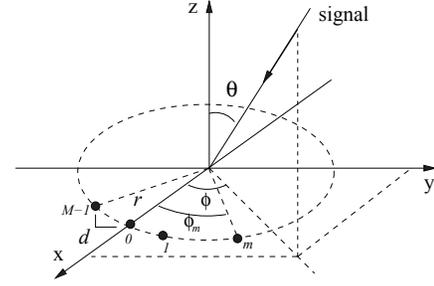
Figure 1: A uniform circular array with  $M$  sensors and a circumferential sensor spacing  $d$  and a radius  $r$ , where a signal impinges from the direction  $(\theta, \phi)$ .
