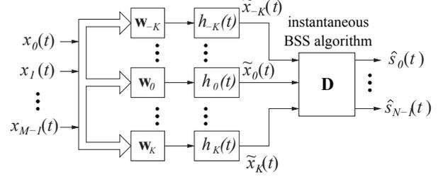
Figure 3: The  $2K + 1$  processing blocks with outputs  $\tilde{x}_k(t)$ ,  $k = -K, \dots, -1, 0, 1, \dots, K$ , followed by an instantaneous BSS algorithm to recover the source signals.
