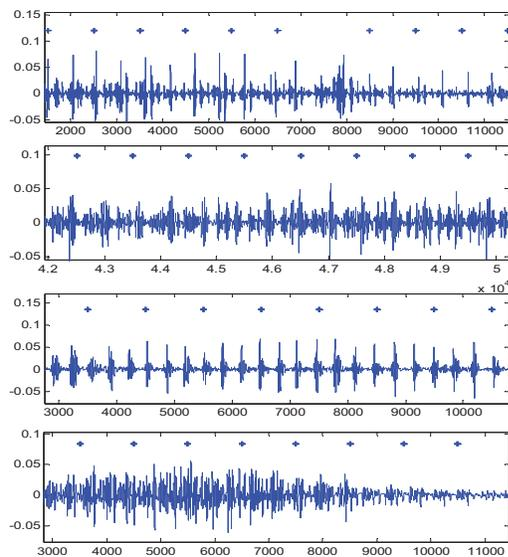
**Fig. 3:** Example of horse's typical footsteps and their recognition: From top to bottom, each plot represents the temporal signal from walk, canter, trot, and gallop respectively. X-axis is sample in 1/1000s. Note blue crosses on top of the signal meaning recognized as horse's footsteps.
