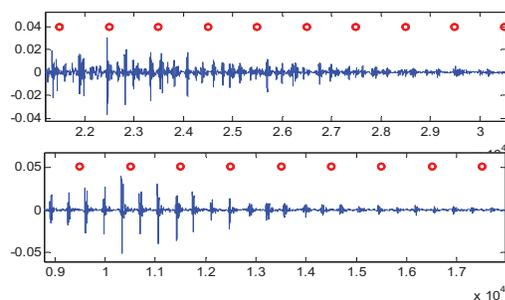
**Fig. 4:** Example of human's typical footsteps and their recognition: The top plot represents the temporal signal from multiple people walking, and the bottom one running. Note red circles on top of the signal meaning recognized as human's footsteps.
