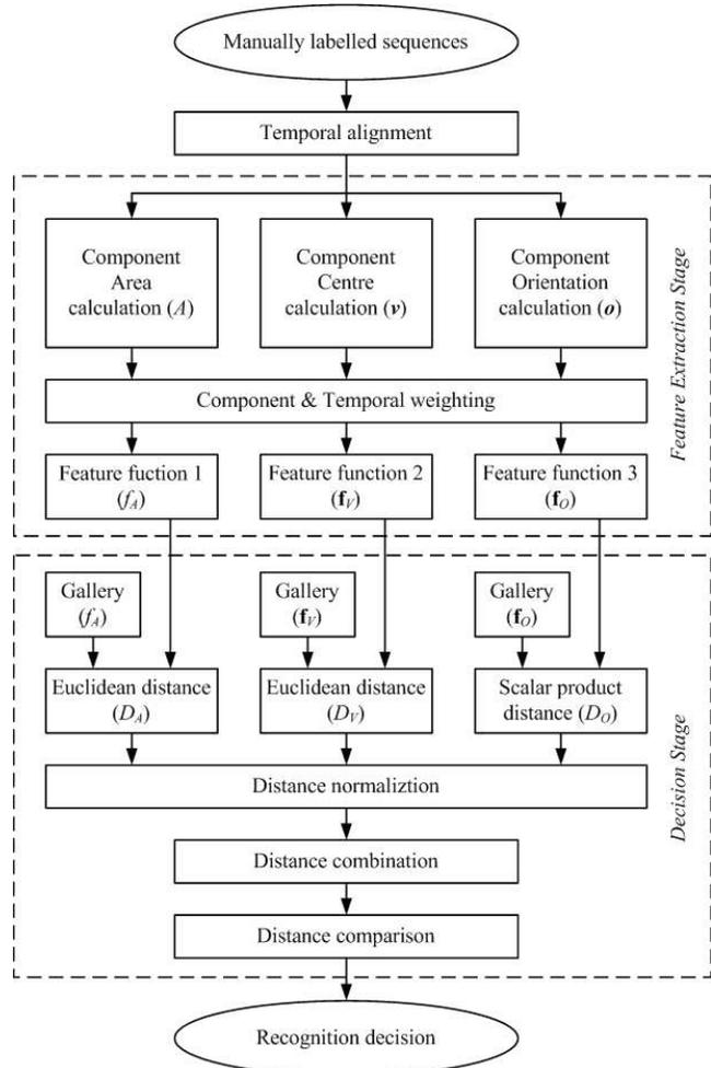
Fig. 2. Block diagram of the proposed algorithm
