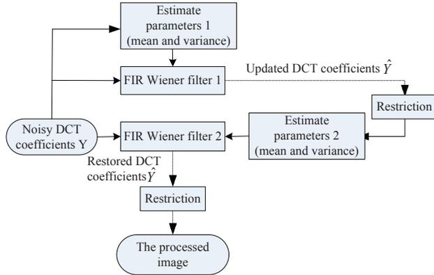
Fig. 3. The proposed dual adaptive Wiener filtering structure
