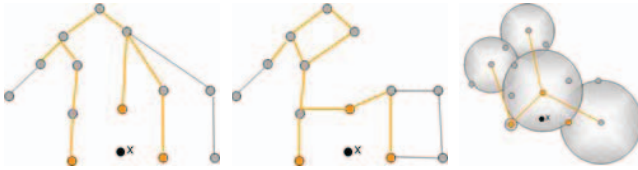
Fig. 5: Comparison of a k -NN ( k=3 ) query in three indexing structures. Left: SA-tree; Middle: RNG; Right: MOBHRG.
