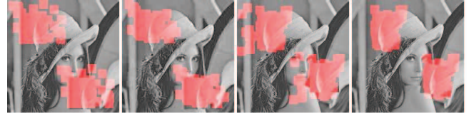
Fig. 3. Shown are the detection results for tampered Lena images. First image has no operation, second saved with JPEG quality of 20, the copied area in the third image scaled 5% and it is rotated 5° in the forth image.
