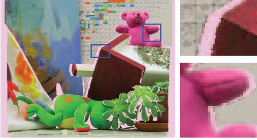
**Fig. 5.** Color bleeding artifacts in the interpolated center image due to the inappropriate baseline interpolation algorithm [2].
