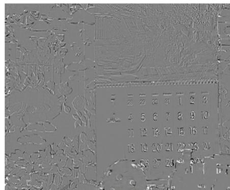
Fig. 1. Motion compensation residual (Mobile sequence at CIF resolution, frame 8 and 10)
