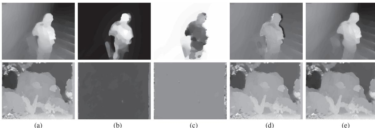
**Fig. 3.** Disparity and motion fields in “Outdoor” (top) and “Aqua” (bottom) stereo sequences: (a) disparity in the previous frame (b) horizontal left motion (c) vertical left motion, (d) initial disparity and (e) final constrained disparity in the current frame.
