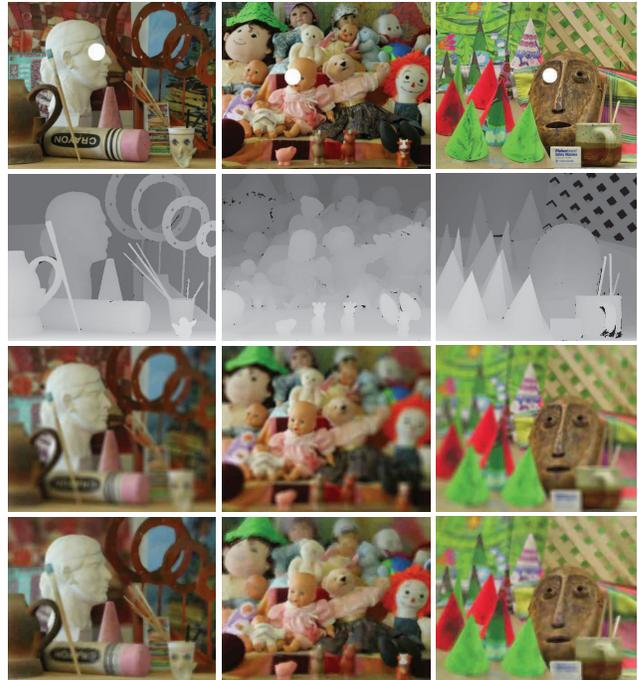
**Fig. 2.** Top: raw images (*Art*, *Dolls* and *Cones*), with our chosen points of interest shown by a white dot. 2<sup>nd</sup> row: associated disparity maps. 3<sup>rd</sup> row: foveation filtered, JPEG-encoded test images for mean blur 10. Bottom: images using distance blurring.
