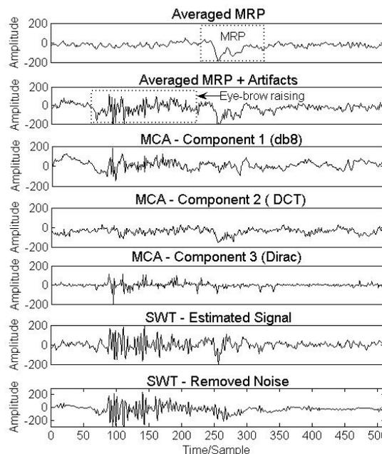
**Fig. 2.** Decomposition of the averaged MRP contaminated by muscle artifacts (eye-brow raising) using MCA and SWT.
