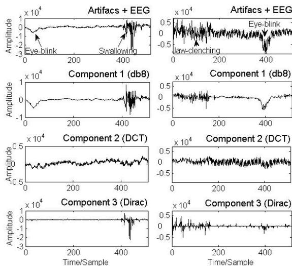
**Fig. 1.** Decomposition of the EEG signals contaminated by artifacts caused by eye-blink and swallowing (column 1), and power line interference, jaw-clenching and eye-blink (column 2) using MCA.
