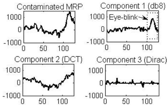
**Fig. 3.** Decomposition of the single-trial MRP contaminated by eye-blink artifacts using MCA.
