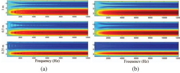
**Fig. 6.** Analytically simulated HRTFs at  $r = 1.0$  m (top plots) and the reconstructed HRTFs at  $r = 0.5$  and  $r = 0.25$  m (a) compared to the reference (b). The horizontal axis is frequency and the vertical axis is azimuth from  $[-\pi, \pi]$ .
