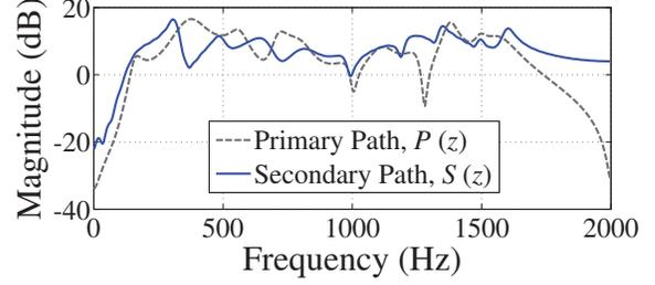
Fig. 4. Magnitude response of acoustic paths used in computer simulations.
