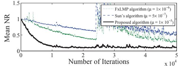
**Fig. 6.** Curves for noise reduction (NR) averaged over 25 realizations for various algorithms.
