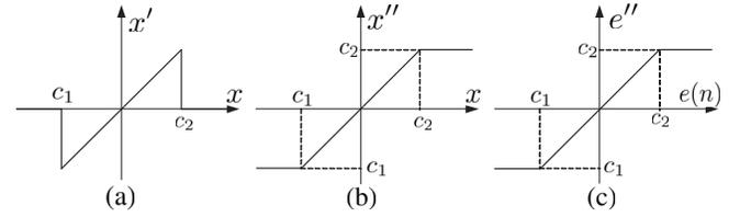
**Fig. 3.** Transformation for (a) reference signal in Sun's algorithm, (b) reference signal in proposed method, and (c) error signal in proposed method.
