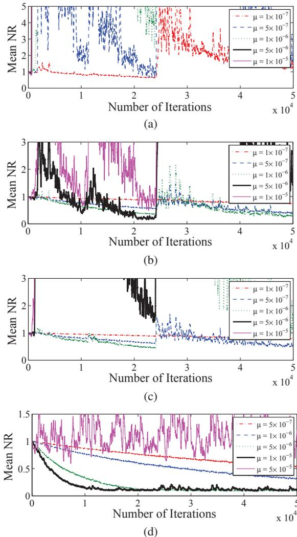
**Fig. 5.** Curves for noise reduction (NR) averaged over 25 realizations for each value of step-size shown in legend. (a) FxLMS, (b) FxLMP, (c) Sun's and (d) proposed algorithm.
