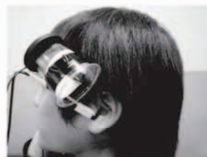
Fig. 7. Head-mounted ANC system used in this experiment.
