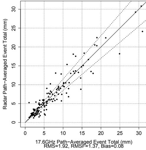
obtained from the 17.6 GHz link, while on the  $y$ -axis is the corresponding radar-based estimate using a weighted combination of the values recorded over 14 cells of the radar’s 2 km  $\times$  2 km Cartesian grid. The dotted lines correspond to  $\pm 15\%$  of the link value. On average there is negligible bias, though the agreement between the estimates is not as close as had been found with the dual-frequency procedure.
