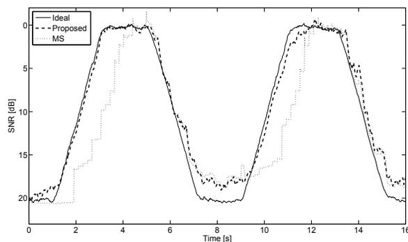
**Fig. 1.** Noise tracking performance of the proposed method and MS on speech contaminated with highly-nonstationary white Gaussian noise. The noise level changes at a maximum rate of 10 dB/s.
