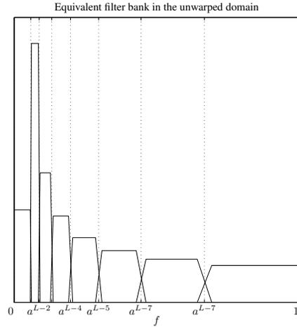
**Fig. 6:** Schematic representation of the equivalent filter bank in the unwarped domain, normalized axis, corresponding to a  $L$ -band uniform filter bank in the warped domain with  $L = 8$ , according to the map depicted in fig. 5.
