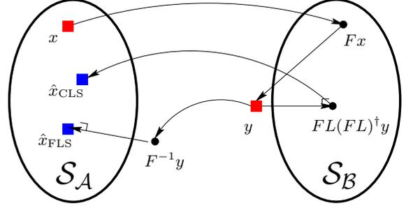
**Fig. 2.** Graphical representation of the estimator operations. Set  $\mathcal{S}_A$  represents the convex set of bandlimited signals. Set  $\mathcal{S}_B$  represents the convex set of signals which can be written as  $\mathbf{F}s$ , where  $s \in \mathcal{S}_A$ .
