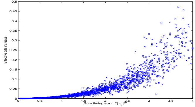
**Fig. 4.** Effective bit increase of estimator CLS over FLS in a 16-ADC system with  $\omega_c = 0.75\pi$ . System timing skew is measured by  $\sum |\tau_i|/T$ . Each x on the plot represents a random set of skews.
