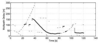
**Fig. 3**. Example of multipath channel on range 4 with weak (dash-dotted) and strong (bold) echoes. Estimated echo tracks (grey) shown if  $p(e_{2,4,k}|\mathbf{Z}_k) > 0.8$ .
