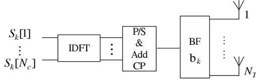
**Fig. 2.** Block diagram of the post-IDFT beamforming transmitter
