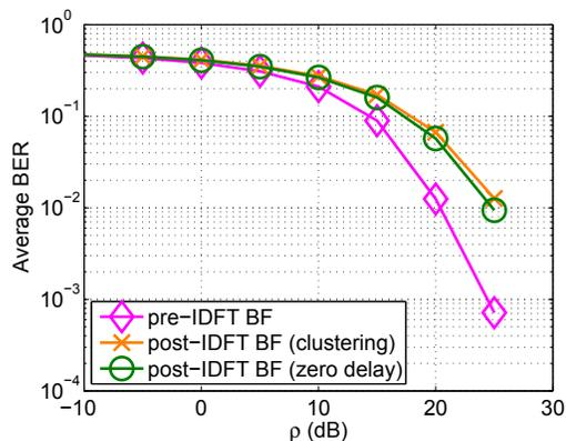
**Fig. 5.** BER comparison for SINR-Max cooperative beamforming for MIMO-OFDM with  $N_c = 64$  and  $L = 16$
