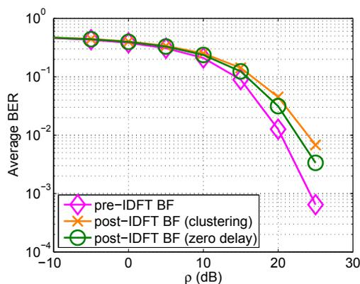
**Fig. 4.** BER comparison for SINR-Max cooperative beamforming for MIMO-OFDM with  $N_c = 64$  and  $L = 6$
