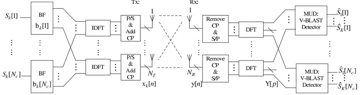
**Fig. 1.** Block diagram of a multiuser MIMO-OFDM SDMA system with the pre-IDFT beamforming
