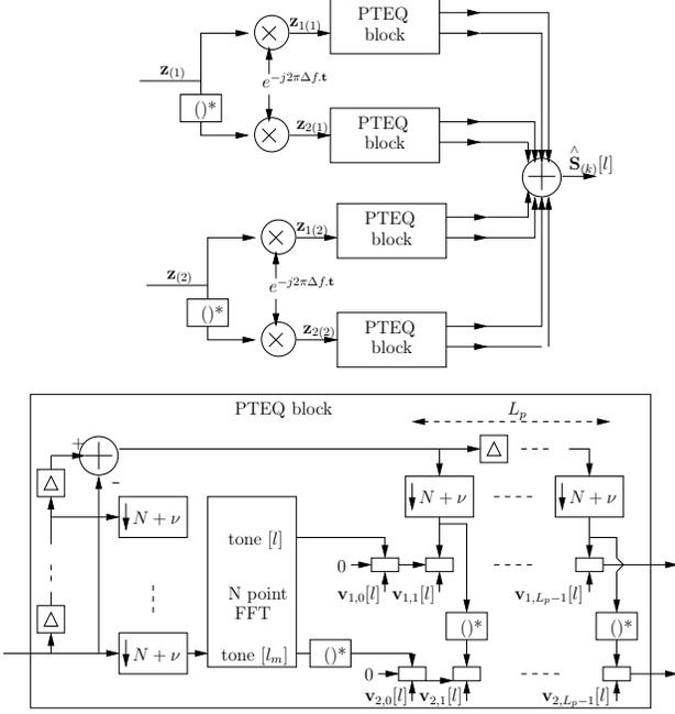
**Fig. 1.** PTEQ compensation for 2x2 MIMO OFDM system
