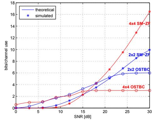
**Fig. 2.** Spectral efficiencies achieved by OSTBC and SM-ZF in a spatially correlated Rayleigh fading channel with  $\rho = 0.5$
