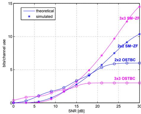
**Fig. 1.** Spectral efficiencies in an i.i.d. Rayleigh fading channel
