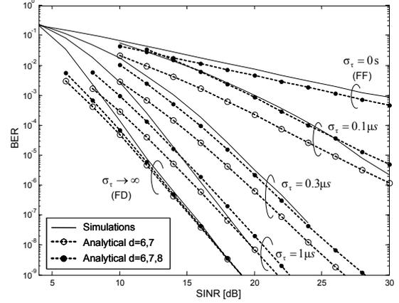
**Fig. 2.** Performance of a single-antenna WiMax system with QPSK modulation. The BER is evaluated at the output of the CC decoder.
