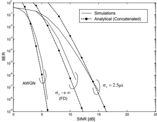
**Fig. 3.** Performance of a single-antenna WiMax system with QPSK modulation. The BER is evaluated at the output of the RS decoder.
