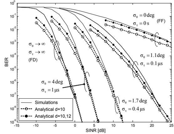
**Fig. 4.** Performance of a 4-antenna WiMax system with 16-QAM modulation. The BER is evaluated at the output of the CC decoder.
