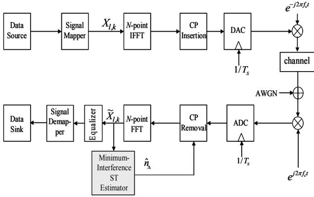
Fig. 1. A simplified OFDM system model.
