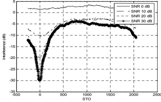
Fig. 3. Interference detected by the minimum-interference estimation of (13).
