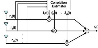
Fig. 1. General Antenna Combining Framework
