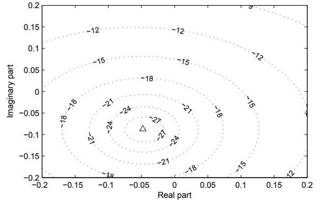
Fig. 1. A contour plot of the cost function  $\mathcal{J}(\hat{\alpha})$  in dB. The desired IQ parameter  $\alpha$  is indicated by  $\Delta$ .
