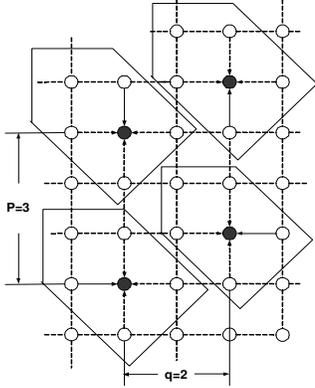
**Fig. 1.** A large network on square grid is partitioned into subnets. Here,  $p = 3$ ,  $q = 2$ ,  $L = 6$  and  $n_0 = n_j = 4$ .
