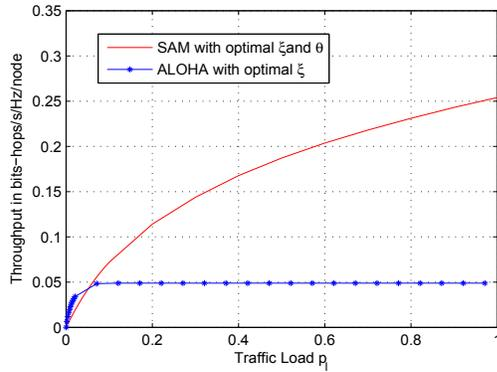
**Fig. 2.** Throughput of SAM and ALOHA versus load probability.  $SNR = P/\sigma^2 = 10dB$ .
