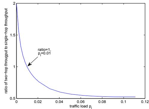
**Fig. 4.** Ratio of distance weighted throughput of different transmission ranges: 2-hop range over 1-hop range.
