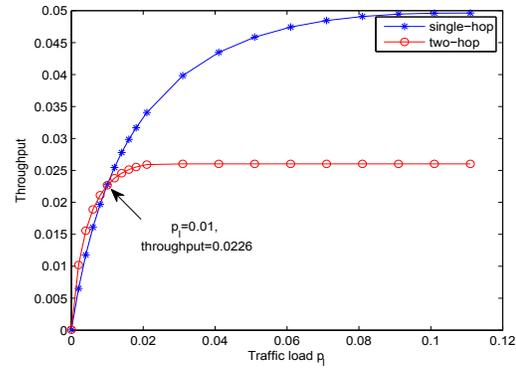
**Fig. 3.** Distance weighted throughput of ALOHA with different transmission ranges: 1-hop range and 2-hop range.  $P/\sigma^2 = 10dB$  for 1-hop range, and  $2^{-\alpha}P/\sigma^2 = 10dB$  for 2-hop range.  $\xi = \xi_{opt}$  and  $p_t = p_{opt}$ .
