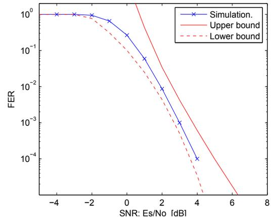
Fig. 3. Lower and upper bounds on the FER of turbo-equalized Proakis-B channel with packet size  $N = 256$  using convolutional code (7,5) in comparison with simulated results.
