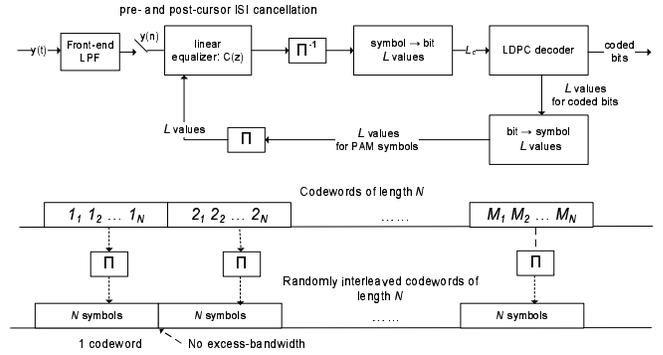
Fig. 2. Iterative linear equalizer from [7].
