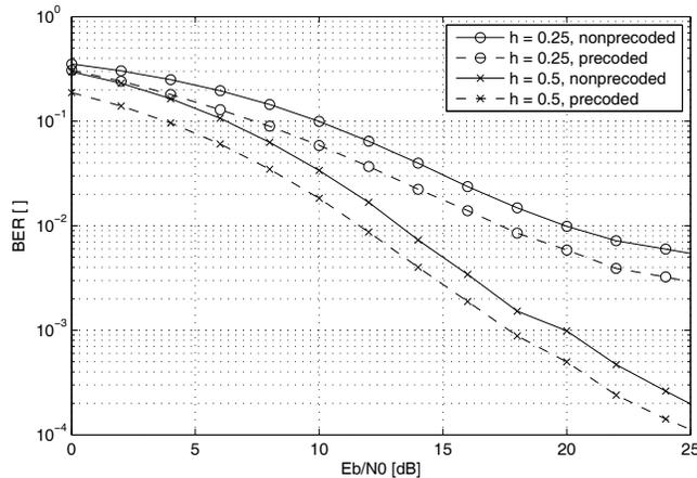
**Fig. 3.** BER performance of the  $3RC$ ,  $h = 0.5$  and  $h = 0.25$  schemes in a 60 GHz environment, both nonprecoded (solid lines) and precoded (dashed lines).
