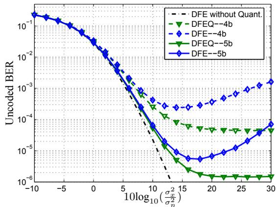
**Fig. 2.** DFEQ vs. the conventional DFE, QPSK modulation with  $M = 10$ ,  $N = 10$ , 4- and 5-bit uniform quantizer, with  $\rho_q = 0.011535$  and  $\rho_q = 0.00349$ , respectively.
