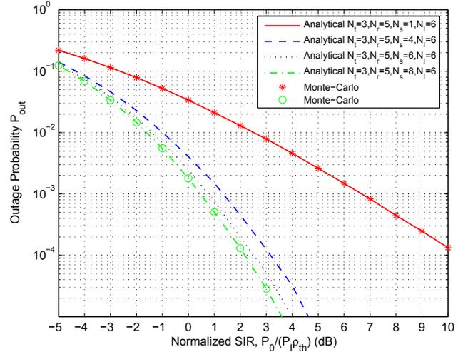
**Fig. 1:** Outage probability of RP-MIMO channels for various  $P_0/(P_{\mathcal{I}}\rho_{\text{th}})$  without noise.
