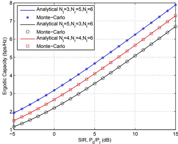
Fig. 3: Ergodic capacity of keyhole channels for various  $SIR = P_0/P_{\mathcal{I}}$ .
