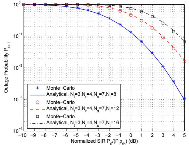
**Fig. 2:** Outage probability of RP-MIMO channels for various  $P_0/(P_{\mathcal{I}}\rho_{\text{th}})$  with  $P_{\mathcal{I}}/\sigma^2 = 3$  (dB) and CCIs with unequal power. For the CCIs, we have set  $\sum_{i=1}^{N_{\mathcal{I}}} P_i = N_{\mathcal{I}}$  and  $P_i = \frac{2i-1}{N_{\mathcal{I}}}$ , for  $i = 1, \dots, N_{\mathcal{I}}$ .
