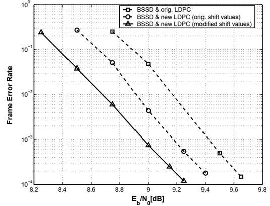
**Fig. 5.** Frame-error rate performance of bounded SSD with original and newly designed block-structured LDPC codes (old and modified shift values); Rayleigh fading channels, 4x4 16-QAM, 4 outer iterations, 15 inner LDPC iterations.
