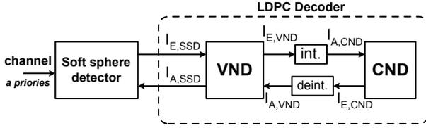
**Fig. 1.** Tracking of *a priori* and extrinsic mutual information; iterative detection-decoding receiver with inner SSD and outer LDPC decoder.
