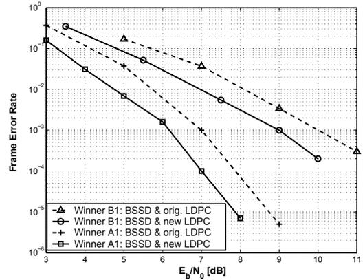
**Fig. 6.** Frame-error rate performance of bounded SSD with original and newly designed block-structured LDPC codes; Winner A1-NLOS and Winner B1-NLOS channels, 4x4 16-QAM, 4 outer iterations, 15 inner LDPC iterations.
