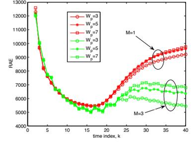
**Fig. 3.** RAE plots for  $M = 1$  and  $M = 3$  and different values of  $W_p$  with  $\rho_{T,m} = 289(1 - \epsilon)^m$ .
