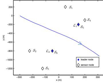
**Fig. 1.** Simulation Scenario for the LNS problem.  $\{S_1, S_2, S_3, S_4, S_5, S_6\}$  are the sensor nodes and  $\{L_1, L_2\}$  are the leader nodes.
