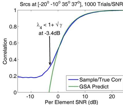
**Fig. 3.** Comparison of predicted and observed projection of the 4th sample eigenvector onto the true signal subspace. The correspondence between the observations and the predictions above  $\lambda_4 < 1 + \sqrt{\gamma}$  is accurate even at small array sizes such as the  $M = 20$  array.
