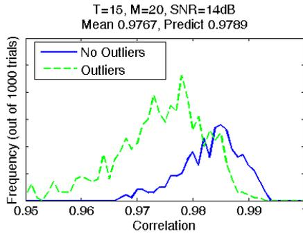
**Fig. 2.** Projection of 4th true eigenvector onto the sample signal subspace.
