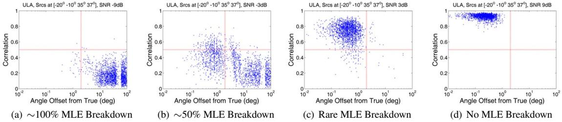
**Fig. 4.** Distribution of DOA estimation errors versus projection  $\mathbf{e}_j^H \hat{\mathbf{E}}_S \hat{\mathbf{E}}_S^H \mathbf{e}_j$  for worst error in multiple source scenario on 20-element uniform linear array with  $T = 15$  training samples. As with the single source case, the projection of the true eigenvector onto the sample signal subspace is a necessary but not sufficient condition for breakdown to occur.
