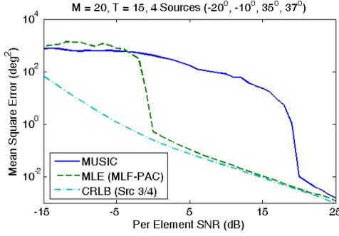
**Fig. 1.** Multiple-source estimation on a 20-element uniform linear array with  $T = 15$  training samples for MUSIC and MLE.
