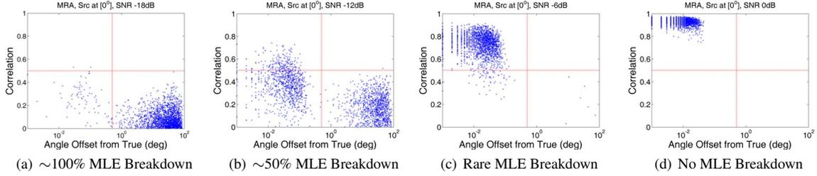
**Fig. 3.** Distribution of DOA estimation errors versus projection  $\mathbf{e}_j^H \hat{\mathbf{E}}_S \hat{\mathbf{E}}_S^H \mathbf{e}_j$  for a single target scenario on 18-element minimum redundancy array with  $T = 14$  training samples. As SNR is increased, the projection approaches unity, and the estimation accuracy improves. Note, however, that trials with low projection values still frequently have low estimation errors.
