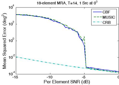
**Fig. 2.** MSE for MUSIC and MLE (CBF) DOA estimation on a 18-element minimum redundancy array with 1000 trials/SNR step. Note that MUSIC delivers essentially the same performance as MLE in this circumstance, as expected for single sources.
