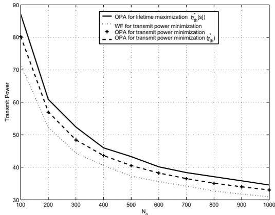
**Fig. 1.** Average power consumption vs. network size ( $D_T = 0.001, \sigma_n^2 = 0.01, \sigma_w^2 = 0.1$ ). The performance of OPA (dotted curve) was evaluated with the approximate threshold  $\gamma_{th}^*$  in (12), whereas markers on that curve (+) show results with the true optimal threshold computed numerically.
