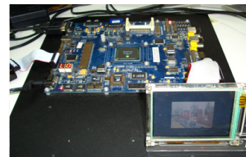
Fig.10. Verification of H.264 decoder on Faraday FIE8100 development board
