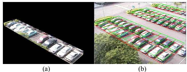
Fig. 1(a) An image partition for a row of parking spaces in the image. (b) The projection of 3-D cubes onto the 2-D image forms the top (green) and bottom (red) lines of the parking spaces.
