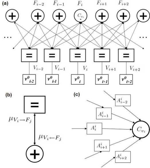
**Fig. 1.** Factor graph representation of Active contours. (a) Bipartite graph AC FG encodes  $\mathbf{A}$ . Variable node  $V_i$  is square equals with initial condition  $\mathbf{v}^0$ . Composite function node  $F_j$  is circle plus. (b). Bidirectional edge update (c). Structure of the composite plus node.
