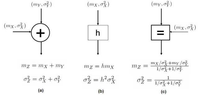
**Fig. 2.** Gaussian message update rules (univariate). (a) Soft plus (b) Product gate (c) Soft equals
