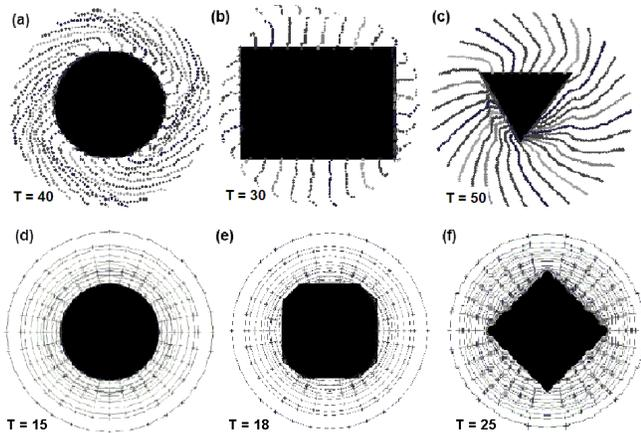
**Fig. 3.** Shape detection using Active contours ( $T$  is the number of iterations required for convergence): (a), (b), (c) using Dynamic programming (d), (e), (f) Message passing algorithm
