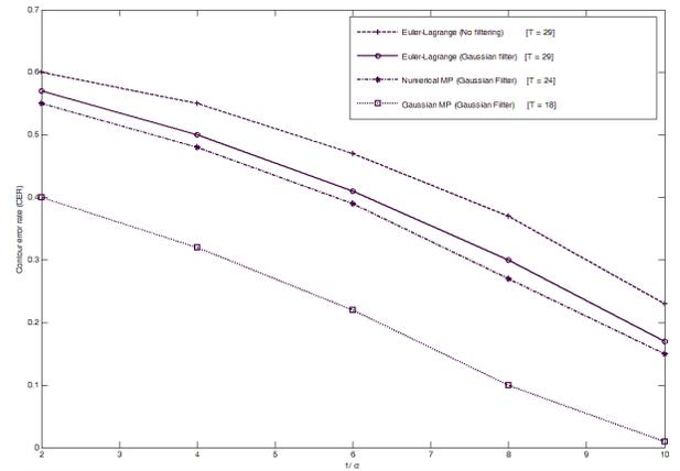
**Fig. 4.** Contour error rate (CER) for varying (Gaussian) noise levels ( $1/\sigma$ ) and Mean number of iterations for convergence ( $T$ ). Contour size = 50. Compared algorithms are Euler-Lagrange (with and without Gaussian filtering), Numerical Message passing, Gaussian Message passing (with filtering)
