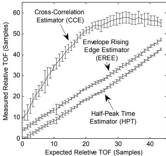
**Fig. 5.** Relative measured vs. expected TOF for the three estimators.
