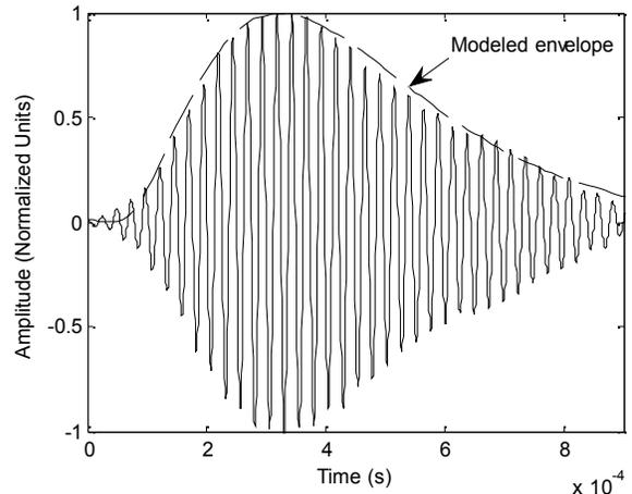
**Fig. 3.** Reference signal with modeled envelope modeled as in equation 4.
