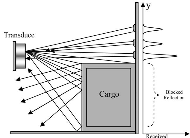
Fig. 1. Return paths of an ultrasound pulse in a shipping container environment.
